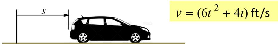
The van shown moves in a straight line such that for a short time its velocity is defined by  $v = (6t^2 + 4t) \text{ ft/s}$ . Knowing that  $t$  is measured in seconds, answer the following:
